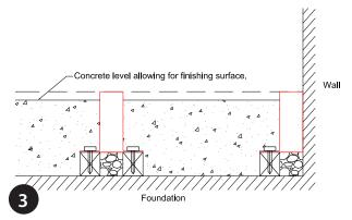
Ensuring housing end caps and housing cover is installed, pour concrete or floor material as required. If finished floor is tiled, grout or mastic can be used to fill gap between housing and finished floor. Ensure that adequate drainage is allowed.
