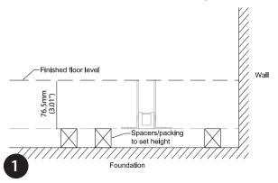
Fix down spacers/packing as required to set installation height of product, ensuring top of product will be level with finished floor level. Ensure that spacers/packing allows adequate drainage.
